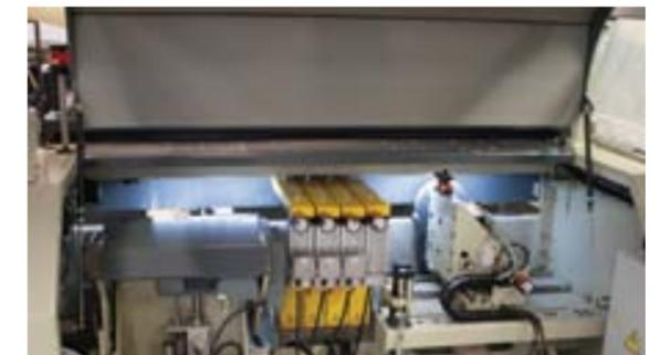
Cross-cutting unit for exact cutting to length, four drilling units, and the milling unit for the fingerjoints
