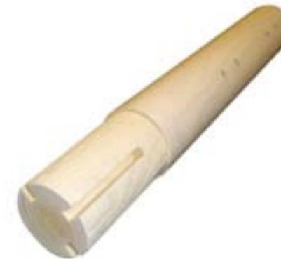
Holes for dowels and milled slots in round workpieces.
