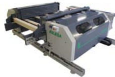
The workpieces are stopped and exactly positioned in every step. After processing, the chain conveyor leads them to the next station.
