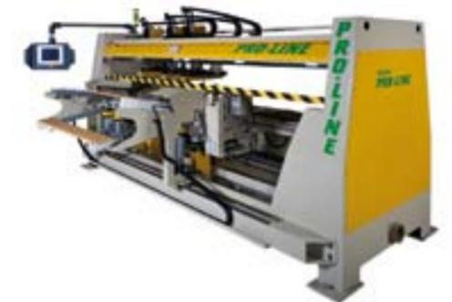
The basic version is designed with a special in- and outlet for the components as they are placed side by side. The components pass through the machine very gently and are handled without any scratches. Resetting the drill groups is done easily and precisely with the magnetic positioning system. When the Pro-line is being fed from other machinery, the pieces are being transported on a conveyor system and transferred crossways into the drilling machine.
