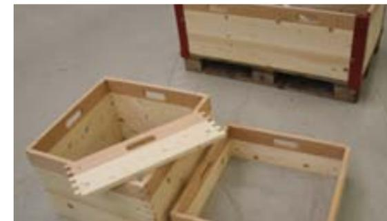
Pallet frames with finger joints, milled handle-holes and insert-nuts, processed in one operation, ready for corner mountings
