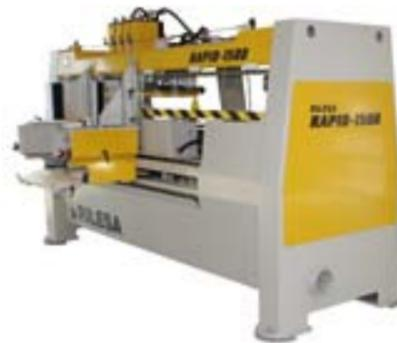
The Rapid machines have a special throughput system where the components are moving in a half circle and returning to the operator on a return conveyor. The Rapid machines are well suited for automation and linking with other machines.
