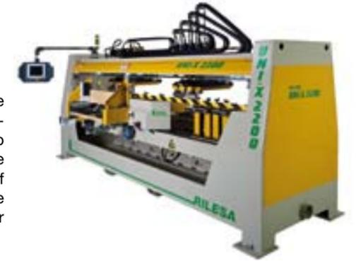
It is possible to reset the machine in minutes, all data regarding drill heads, tools, position in x, y and z direction etc. are stored in the control unit. A digital measuring system combined with a lightsignal guides the operator to position the drill groups in the x-direction. During production the machine continuously controls the position in x-direction to reduce faults.
