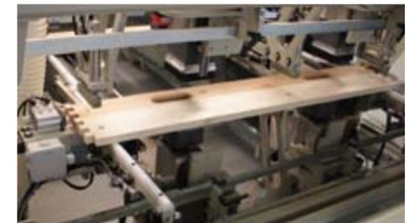
In the last step, four milling units are processing the handle holes in the frame sides from the top and from below
